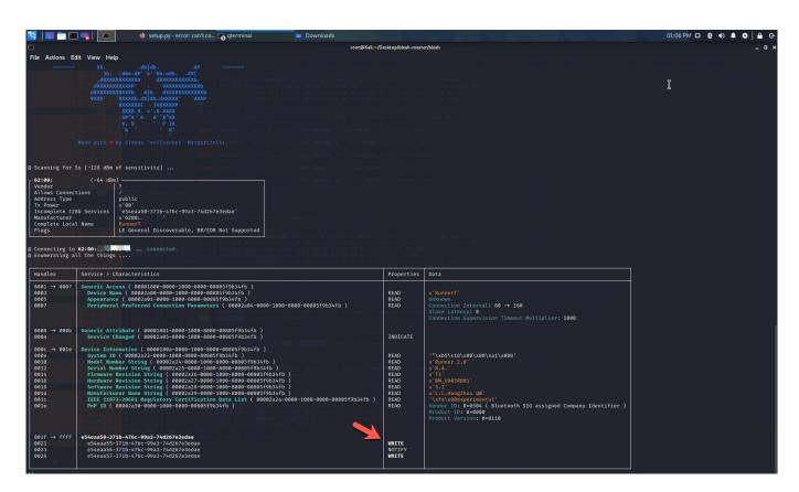
After seeing the WRITE feature in the e54eaa57-371b-476c-99a3-74d267e3edae characteristic information, I sent the bleah -b "62:00:xx:xx:xx:xx" -u "e54eaa57-371b-476c-99a3-74d267e3edae" -d "0x01000000002603" command to the treadmill using bleah and saw that the treadmill started!
