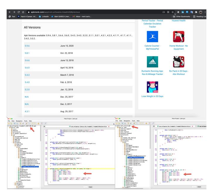
When I quickly looked at the source code, the startTreadmill(long delayMillis) function was called to start the treadmill, then the mBleHelper.writeCommand(getControlCommand(1, 0, 0), delayMillis) function was called, and finally, the getControlCommand(int mode, int speed, int slope) function was called, which creates the 7-byte packet to be sent to the treadmill.
