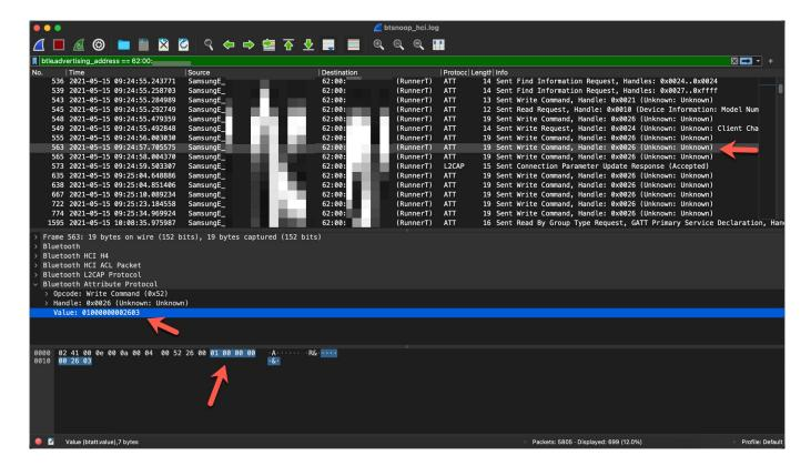
Next, I sent the treadmill the commands Hold/Pause~(05000000002a07), set speed to 9 km/h (035a000000825b), set speed to 5.2 km/h (03340000005c39), and Stop (02000000002704) and saw the other values in parentheses on WireShark.
