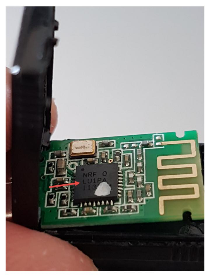
When I opened the receiver, I came across the nRF24LU1PA 2.4 GHz receiver-transmitter chip. When I looked at the document for this chip on the website of the chip's manufacturer, Nordic Semiconductor, the first things that
